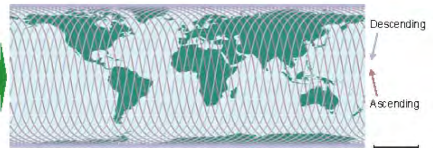
Figure 6. Conceptual diagram of GOSAT observation and the satellite orbits (three days, 44 orbits)
