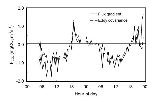
Example of diurnal variation of  $CO_2$  flux measured by the EC-technique and the Flux Gradient technique. From Griffith (2002).
