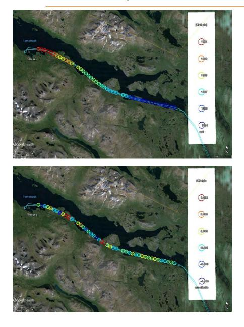
CH<sub>4</sub> concentrations measured during flight No. 2015/7 over lake Torneträsk and the Abisko-Stordalen mire on 13/07/2015.
