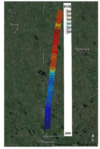
CO<sub>2</sub> fluxes measured during flight No. 2015/2 north of Rovaniemi airport on 23/06/2015.
