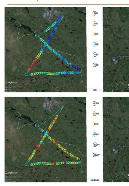
$CH_4$  concentrations measured during flight No. 2015/9 south of Kiruna airport on 13/07/2015.
