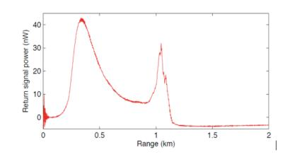
a typical Lidar return measured with the current instrument, where the signal at short range is initially zero due to the shadow effect and increases as the secondary is able to collect more of the photons scattered by the transmitted laser beam. The signal is reduced to zero beyond approximately 1 km by a cloud.
