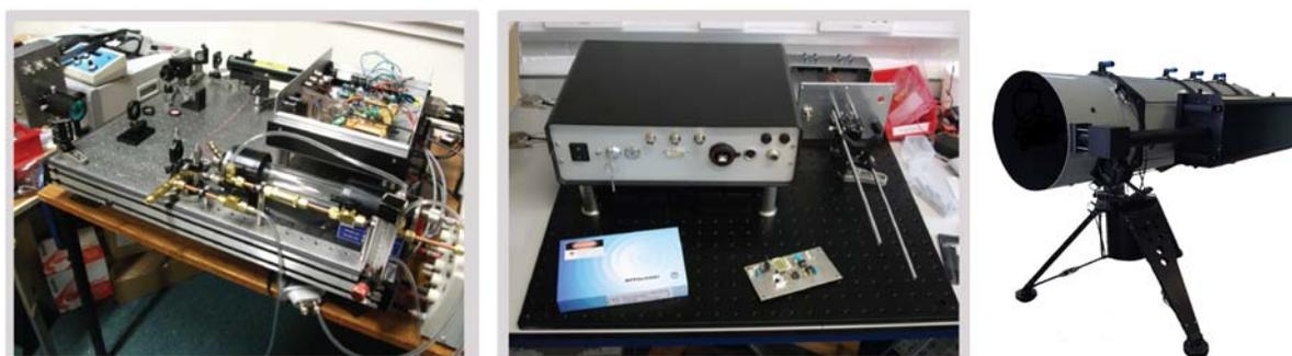
**Figure 1.3.6:** Seed modules ( $\text{CO}_2$  on the left,  $\text{CH}_4$  in the middle) for DIAL of greenhouse gases, a photograph on the right of the Mark 2 DIAL with the laser attached to the tripod-mounted Newtonian telescope
