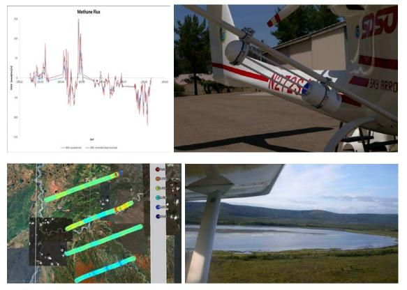
Measurements with the open path licor  $\mathsf{CH}_4$  sensor attached to the wing of the Sky-Arrow airplane.
