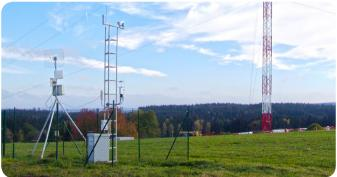
This ICOS Ecosystem station uses a standard methodology (eddy covariance) to monitor matter and energy fluxes between the local agroecosystem and the atmosphere. Micrometeorological and biomass parameters and nutrient contents are measured, too.
